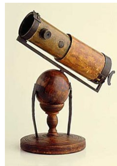
Newton's reflecting telescope
