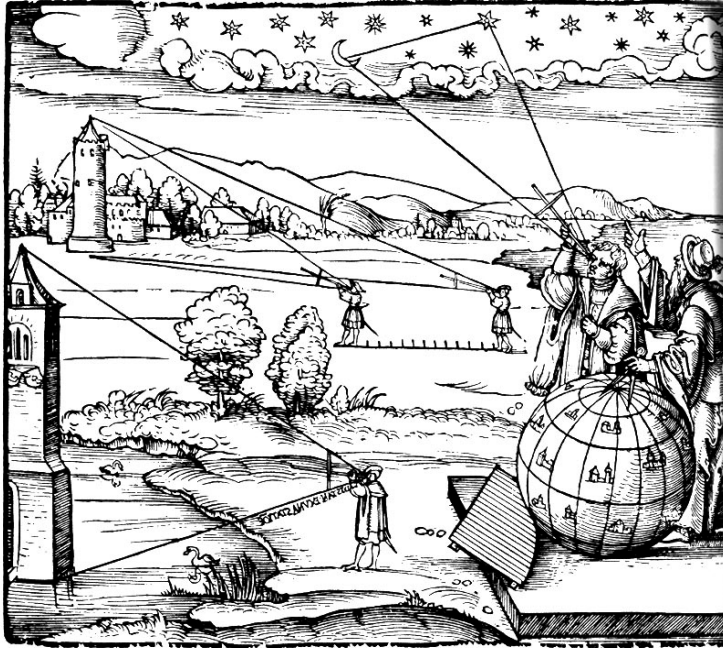
Fig 3: Woodcut from 1533: surveyors are using a cross-staff to measure angles.
