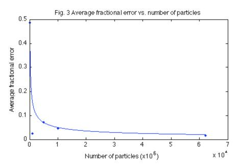
As displayed in Figure 3, the average fractional error decreases rapidly with increasing number of particles. Notably, this is very close to an inverse square root relationship. Therefore, I will postulate that AFE  $\sim 1/\sqrt{(x)}$ . According to this model, increasing the number of random points by a factor of x causes the AFE to decrease by a factor of  $1/\sqrt{(x)}$ . With a significant amount of additional data, it would be possible to test and investigate this relationship.
