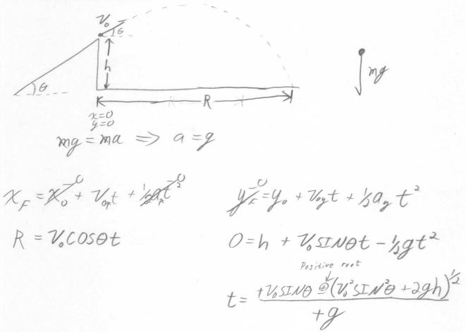
$\left[R = \frac{1}{g} V_0 \cos \left[V_0 \sin \theta + \left(V_0^* \sin \theta + 2gh\right)^2\right]\right]$
