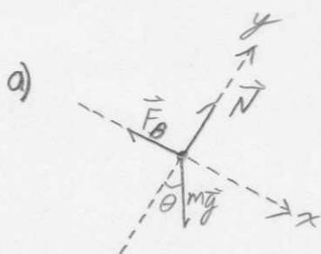
$$\text{In the } x, F_c - mg \sin \theta = 0 \\ \text{to maintain } V = 100 \text{ mph}$$
