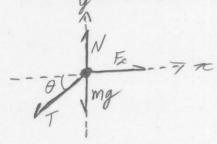
b. Draw a freebody diagram of the ice block. (It's frictionless)
