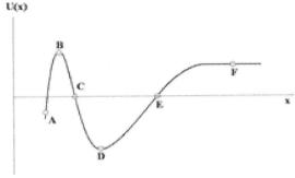
a) At each point indicated, state whether the corresponding force  $F_x$  acting on the particle is positive, negative, or zero.
