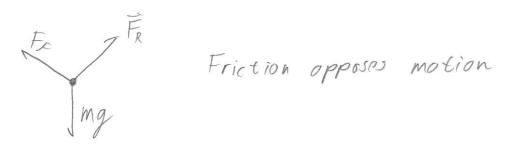
A 30-kg child is seated in a swing of negligible mass. How much horizontal force is required to pull the child and swing aside so that the support rope makes an angle of 32° with the vertical? (The child is held fixed in that position.)
