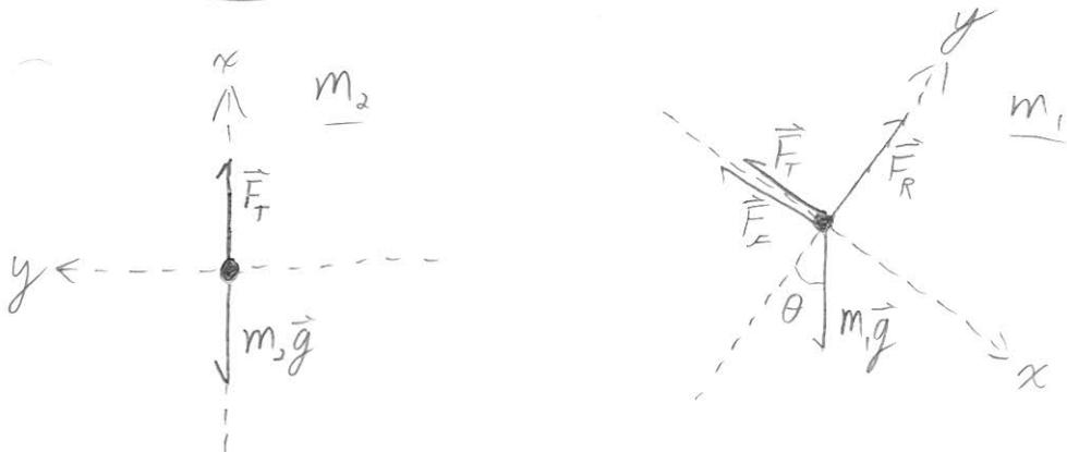
The coordinate systems here are aligned so that the positive  $x$ -axes are in the direction of the acceleration of the block.
