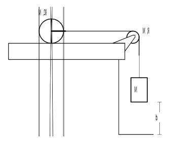
A block of mass M rests on a rough table with  $\mu_k = 0.3$ . A massless string is attached to the block, wrapped around a solid cylinder having a mass M and a radius R, runs over a massless frictionless pulley, and is attached to a second block of mass M that is hanging freely.
