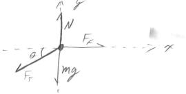
b. Draw a freebody diagram of the ice block. (It's frictionless)
